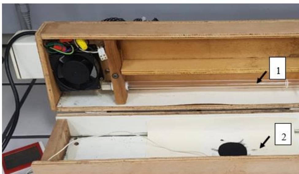
Legenda: 1 – Lâmpada ultravioleta GERMICIDA 25W - GPH846T5VH / HO / 4PSE de 185 nm;
