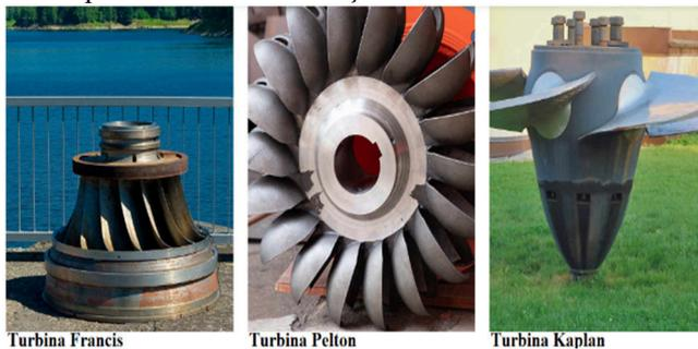
Figura 5: As Três Turbinas (Francis, Pelton, Kaplan)
