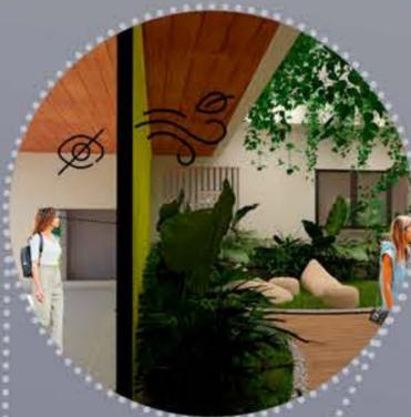
BRISES VERTICAIS FIXOS EM ACM PINTADOS COM TINTA EPÓXI NA COR AMARELA
