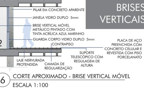
6 CORTE APROXIMADO - BRISE VERTICAL MÓVEL ESCALA 1:100
